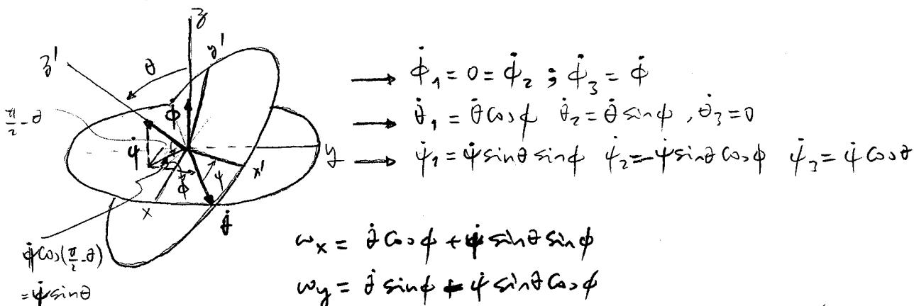
$$\begin{pmatrix} \dot{\theta}_1 \\ \dot{\theta}_2 \\ \dot{\theta}_3 \end{pmatrix} = B^{-1} \begin{pmatrix} \dot{\theta} \\ \dot{\phi} \\ \dot{\psi} \end{pmatrix} =$$
