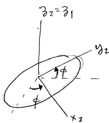
$$\begin{pmatrix} \dot{\theta}_1 \\ \dot{\phi}_1 \\ \dot{\varphi}_1 \end{pmatrix} = IA \sim \begin{pmatrix} \dot{\phi} \\ 0 \\ 0 \end{pmatrix}$$
