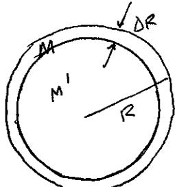
$$\begin{aligned} I_c &= \frac{2}{5}MR^2 - \frac{2}{5}M'(R-\Delta R)^2 & \left\{ \begin{array}{l} M' = \frac{4}{3}\pi S (R-\Delta R)^3 \\ M = \frac{4}{3}\pi S R^3 \\ M_{KAB} = 4\pi R^2 \Delta R S \end{array} \right. \\ &= \frac{2}{5}\frac{4}{3}\pi S (R^5 - (R-\Delta R)^5) \\ &= \frac{2}{5}\frac{4}{3}\pi S \left( R^5 - R^5 + 5 \frac{\Delta R}{R} R^4 + \dots \right) = \frac{2}{15} 4\pi S R^2 \Delta R S R^2 \\ &= \frac{2}{3} M_{KAB} R^2 \end{aligned}$$
